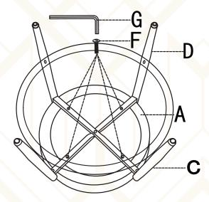
Twist Screw (F) to connect the (A) with (C) and (D).
