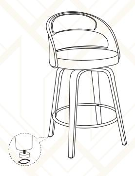
If you feel that the chair is leaning to one side due to an uneven ground, rotate the foot pads to adjust it.
