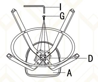
Twist Screw (G) to connect the (A) with (D).
