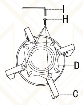
Twist Screw (H) to connect the (D) with (C).
