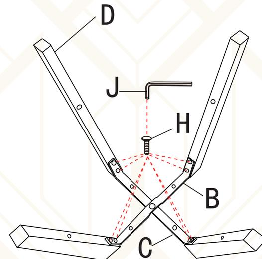
Twist Screw (H) to the (D) with (B) and (C). Only twist (H) into half way in this step.
