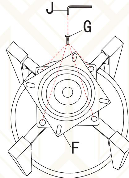
Rotate (F) 45 ° as displayed. Twist Screw
