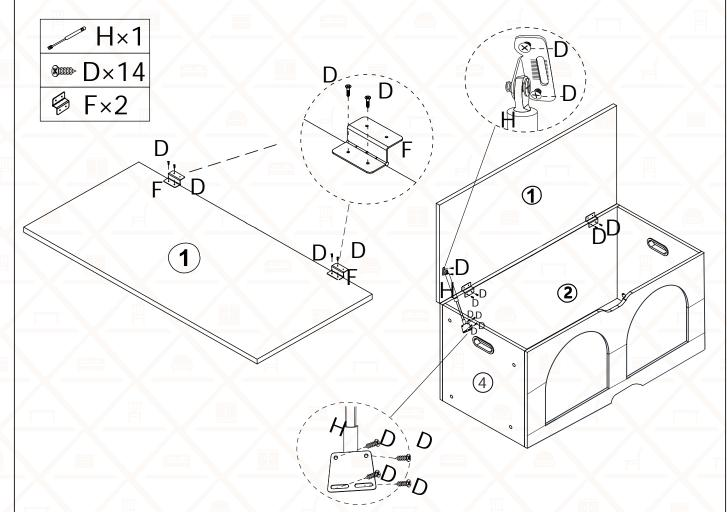
When installing H, first use D\*2 to fix H to board ①, then use D\*4 to fix H to board ④.
